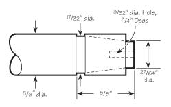
Test fit the cane tip. If the tip is too loose, cut 1/16" from the end of the cane and recut the shoulder of the tenon. Once you are satisfied with the fit, remove the tip, apply a waterproof glue (such as epoxy) to the tenon, and press on the tip. Either wipe off any excess glue with a rag and solvent before it has cured, or sand the cane and tip until the joint is flush after it has cured.
